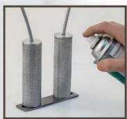
Magnetic flaw detector is based on the method of non-destructive testing used for detecting violations of the magnetic surface of metal structures and structures of ferromagnetic materials.
