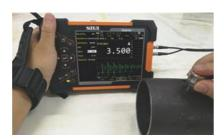
Thickness measurement on pipe
