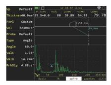
Simulate the weld shape and use the dynamic beam tracking function to assist the user to quickly determine the location of flaws in the weld.
