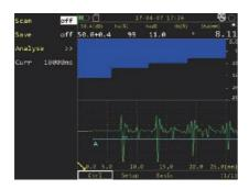
• Based on time interal or encoder, display the measurement readings in B-mode image.
