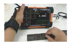
Thickness measurement on step block
