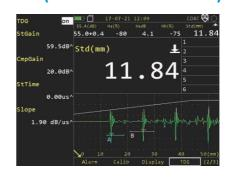
• It can be used for compensating the loss of echo amplitude due to propagation of sound path.
