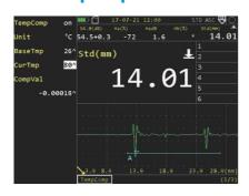
• When there is temperature difference between the calibration block and the detected workpiece, it can be used for temperature compensation.
