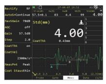
• After setting the coating velocity, through-coating thickness and coating-thickness can be displayed at the same time.
