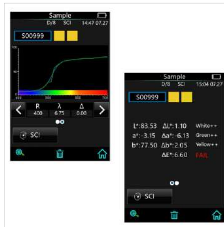
11. Diversified data display Spectrocolorreader CR8 (Professional) can intuitively display reflectance (reflectance at 3 specific wavelength specified by the user), sample chromaticity value, color difference value/graph, pass/fail result, color simulation, color offset and other data. It is convenient to view and also greatly improves the user's work efficiency.
